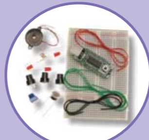
The ECIO student starter kit consists of an ECIO28P, a breadboard, and 13 electronic components which are used with the worksheets.
